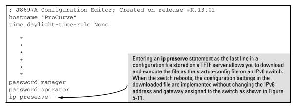
Figure 5-10. Example of How to Enter IP Preserve in a Configuration File
